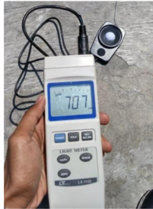
FIGURE 4. Light meter LX used in this experiment to estimate a large amount of sun intensity
