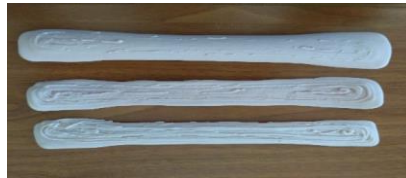
Figure 2: Specimen according to ASTM D638 Type 1.
