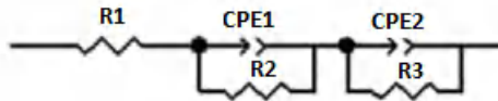
Figure 4. (a)-(c) Nyquist diagram of impedance spectroscopic symmetric cell NBSC+0.5 M SDC|SDC|NBSC+0.5 M SDC in the OPP range between 0.112–0.019 atm at various temperatures and (d) Equivalent circuit used to fit the impedance spectra
