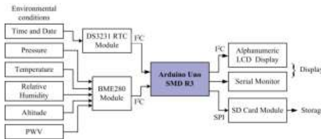
Figure 1. Block diagram of a low-cost weather station development
