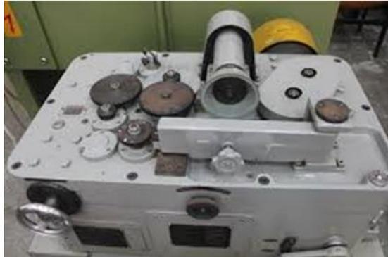
**Gambar 3.8** Alat uji keausan
