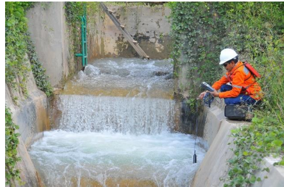
Fig.1 Field measurement of TSS by using portable device (Partech 740)
