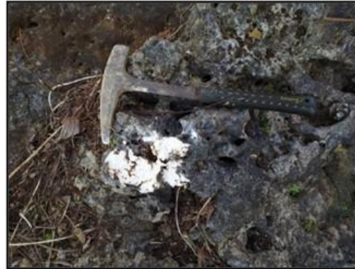
Figure 5. Crystalline limestone in the field showing dissolving hollows (lapies).
