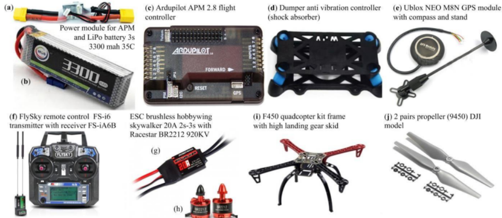
Fig. 4. Materials used for a drone with F450 frame and APM 2.8 flight controllers
