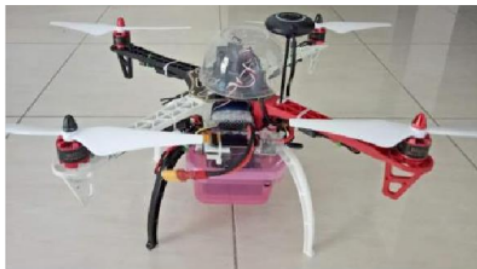
Fig. 6. Assembled drone with an F450 frame and equipped with Arduino meteorological sensors as a payload
