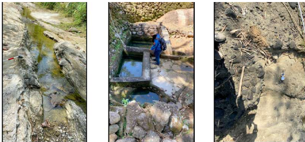
Figure 4. The gauge in Krenceng river, Tambakromo, Ponjong (left). The springs in Grogol village, indicated the structural geology (center). The offset of rock layer (tuffaceous lapillistone and andesitic breccia (right)
