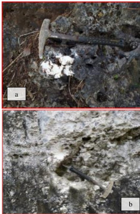
Figure 3 a. Crystalline / Coralline limestone with a lot of lapies and, b. the chalky / clastic limestone with fine to coarse grain size.
