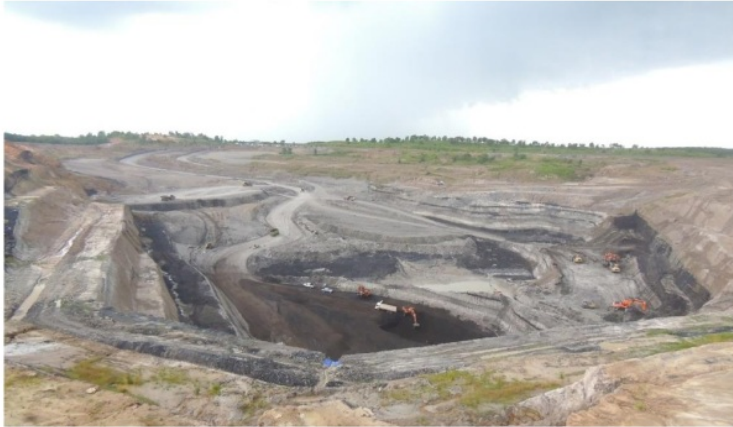
Fig. 13. Mining was completed using undercutting method without any instability issue.
