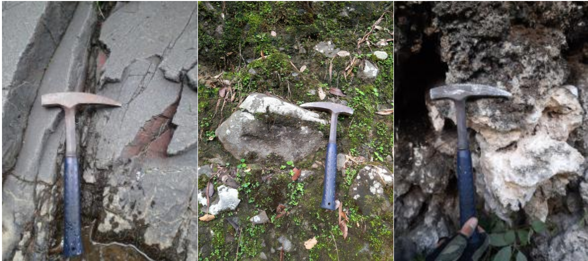
Figure 3. Rock outcrops found in the field: andesite intrusion at Pagerharjo (left); andesite breccia in Sidoharjo (middle); and reef limestones in Purwoharjo (right).
