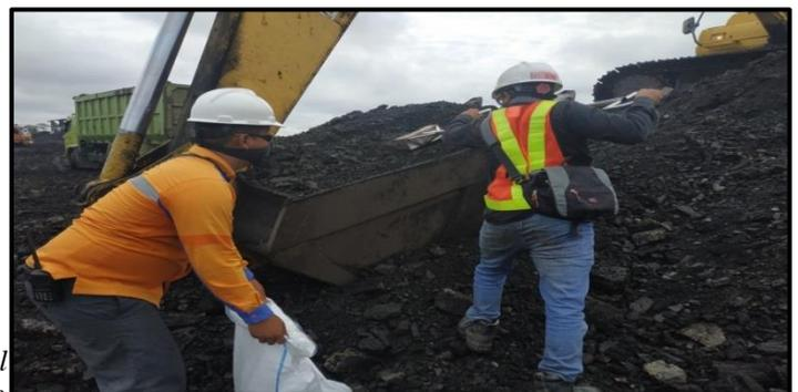
Gambar 4 Pengambilan Sampel *Seam 300 UHS* Di *Stockpile*
