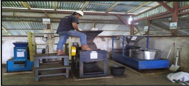
Gambar 6 Proses *Crushing* Sampel Batubara
