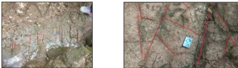
FIGURE 5. (a) Appearance of shear fractures at location 1. (b) Appearance of shear fractures at location 2 near the spring.
