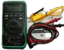
Gambar 4. Multi Tester Digital - Kyoritsu 1011
