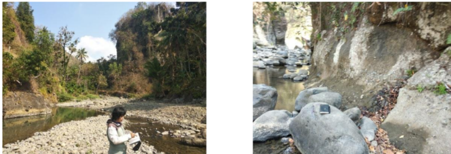
Figure 2. Andesite breccias at the Kahyangan Dam can be groundwater aquifers supported by crack porosity.
