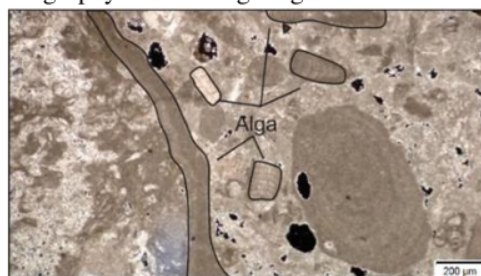
Figure 4. The presence of algae in calcirudite is a marker if rock is formed in the open ocean
