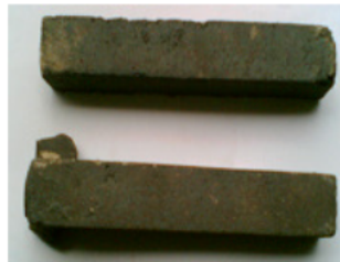
Gambar 1. Ingot coran paduan Fe-2,9Al-0,4C berukuran 30 x 30 x 200 mm
