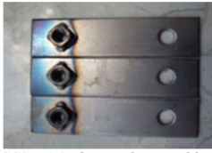
Figure 2. SPCCSD 1.8 plate and Nut weld M6 after welding
