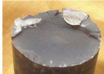
Gambar 1. Permukaan patah poros brine injection pump
