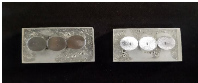
Gambar 3.5. Hasil mounting (resin)
