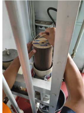
Gambar 1. 8 Melepas Fuel Filter Sparator
