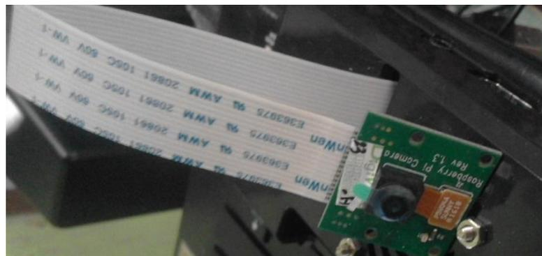
Gambar 2.2. Pi camera raspberry pi
