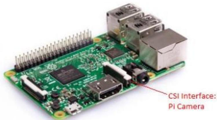
Gambar 2.1. Raspberry Pi 3 Model B
